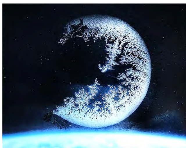
Fig. 2. Photo of frost on the inner side of the outer porthole glass
