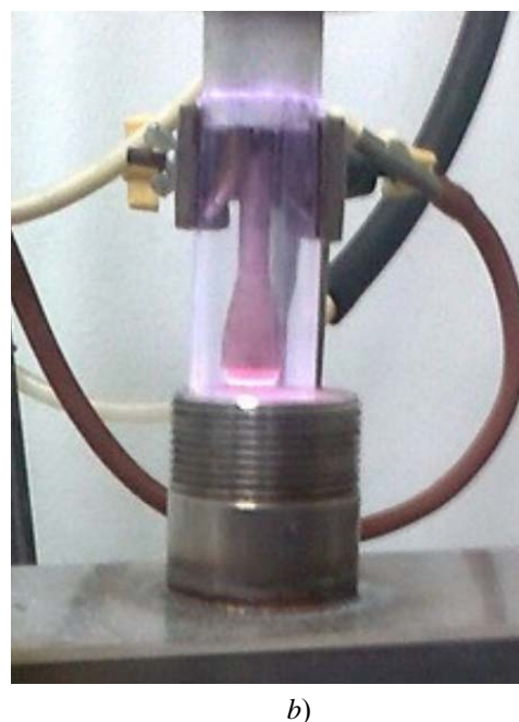
Fig. 1. Scheme of the gas flow former with a bluff body – a vortex-inducing cone (a) and its test prototype during a powder feeding experiment (b)
