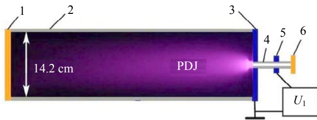
Fig. 1. Experimental setup diagram No. 1 with an inserted photo of the plasma diffusion jet (PDJ) glow obtained at an air pressure of 0.4 Torr and exposure of 0.25 s. 1 and 6 – caprolon flanges; 2 – tube made of ESALUX TX polycarbonate with an outer diameter of 15 cm and wall thickness of 4 mm; 3 – grounded electrode made of duraluminum with a hole for quartz tube 4 with an outer diameter of 21 mm and wall thickness 1.5 mm; 5 – external ring electrode made of steel foil with a width of 10 mm; U_1 – pulse generator with a voltage pulse amplitude at a load of U = +7 kV and frequency f = 21 kHz connected to electrodes 3 and 5
